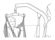
When performing a lift always load the sling bar evenly using both hooks
