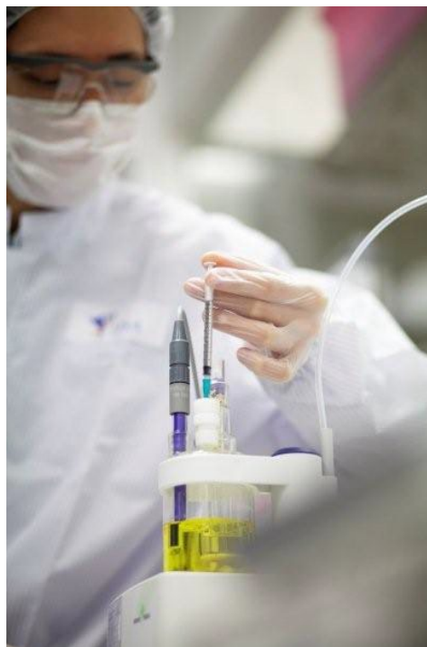
A HSA Chemical Metrology Laboratory staff measuring the moisture level in an alcohol sample for purity assessment
