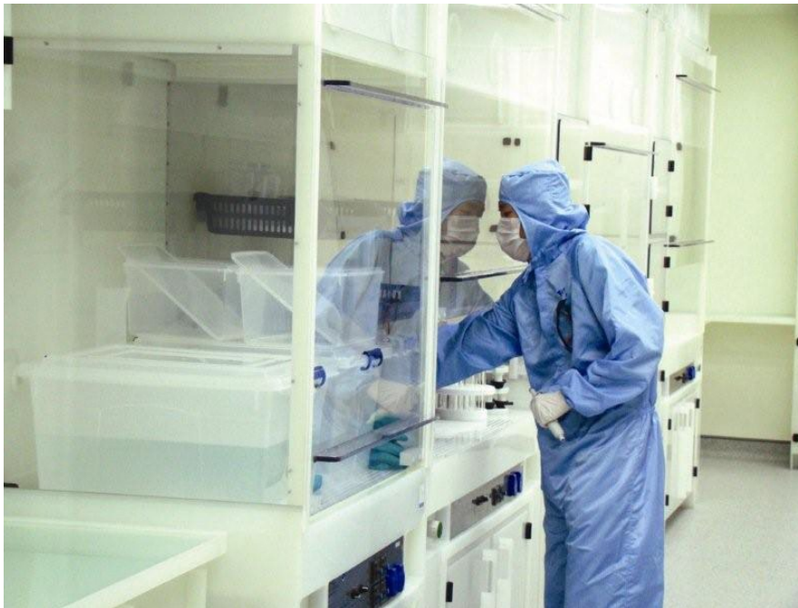
The HSA Chemical Metrology Laboratory conducts sample preparation for inorganic analyses in the “metal free” section
